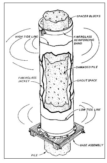
Figure 6-9. Typical preformed fiberglass jacket being used in repair of a concrete pile
