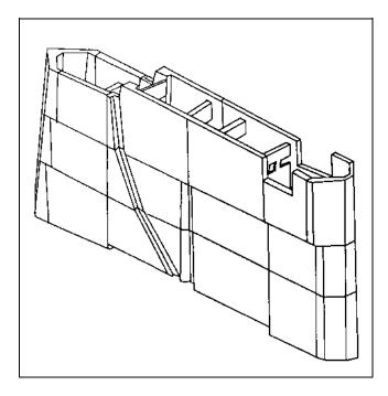
Figure 8-40. Isometric view of gate pier 6, C-1 Dam
