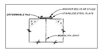
Figure 8-19. Typical plate type waterstop
