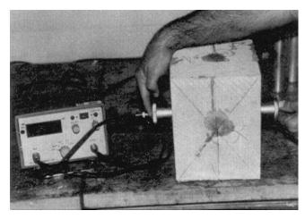
Figure 2-39. Ultrasonic pulse-velocity apparatus
