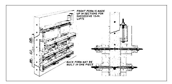
Figure 6-3. Detail of form for concrete replacement in walls after removal of all unsound concrete
