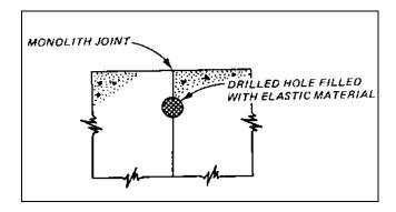
Figure 8-21. Drilled hole with elastic filler
