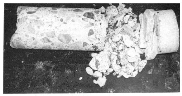
a. Concrete deterioration immediately behind shotcrete overlay
