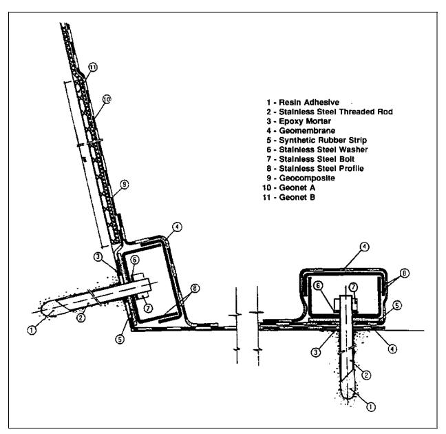
Figure 8-59. Detail of sealing profiles
