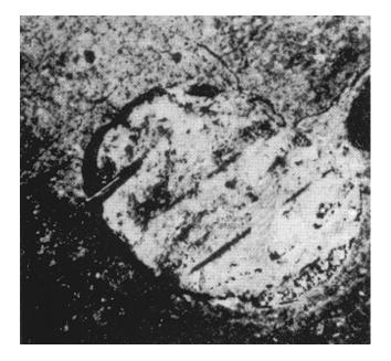
Figure 2-30. Large spall
