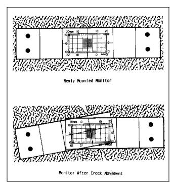
Figure 2-33. Crack monitor
