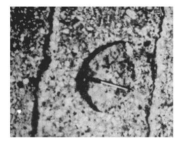
Figure 2-29. Small spall
