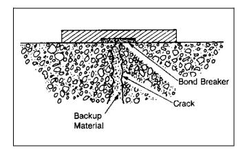
Figure 6-7. Repair of a narrow crack with flexible surface seal
