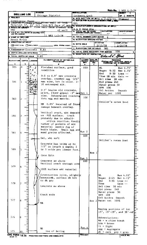
Figure 2-34. Typical information included on a drill log for concrete core
