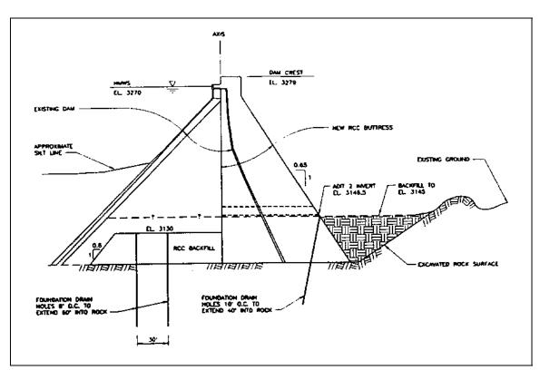
Figure 8-70. Littlerock Dam modification (Bischoff and Obermeyer 1993)
