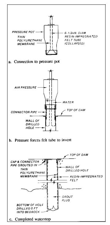
Figure 8-25. Remedial waterstop installation, Pine Flat Dam
