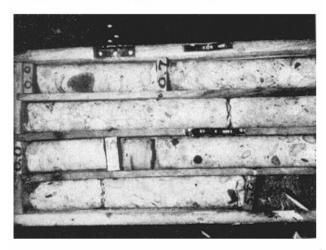
Portions of the core from two drill holes through land chamber wall which was not refaced
