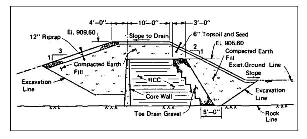
Figure 8-67. RCC spillway section, Boney Falls Dam (Marold 1992)
