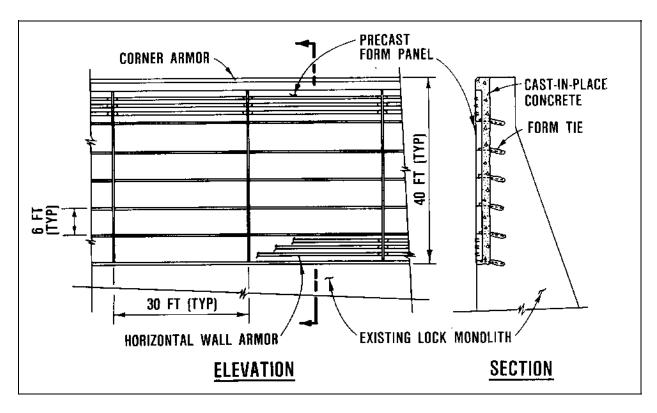
Figure 8-12. Precast concrete stay-in-place forming system for lock wall rehabilitation
