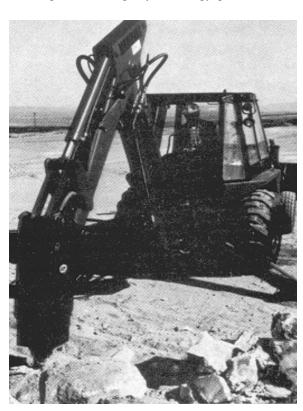
Figure 5-7. Boom-mounted breaker
