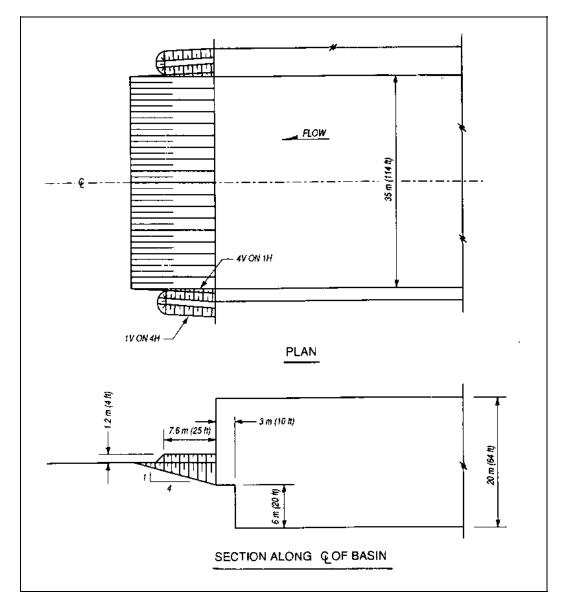
Figure 8-37. Stilling basin wall extension fills, Dworshak Dam
