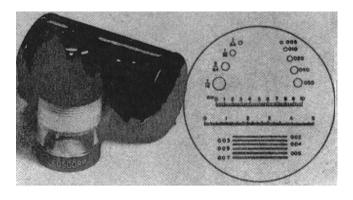
Figure 2-32. Comparator for measuring crack widths
