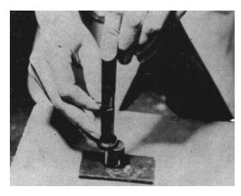
Figure 2-38. Device for measuring length of probe extending from surface of concrete
