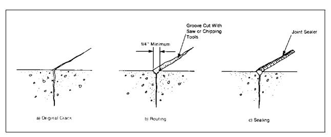
Figure 6-10. Repair of crack by routing and sealing
