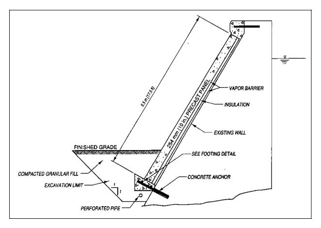
Figure 8-49. Typical repair section, Joliet Channel Wall
