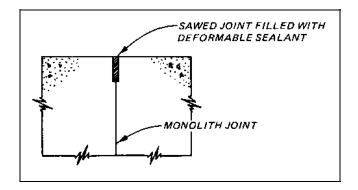
Figure 8-20. Typical sawed joint filled with sealant
