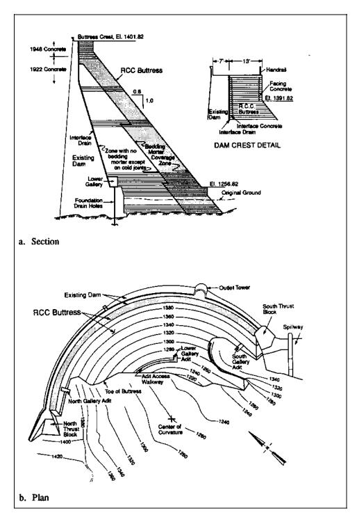
Figure 8-69. Section and plan of modified Gibraltar Dam (Wong et al 1992)
