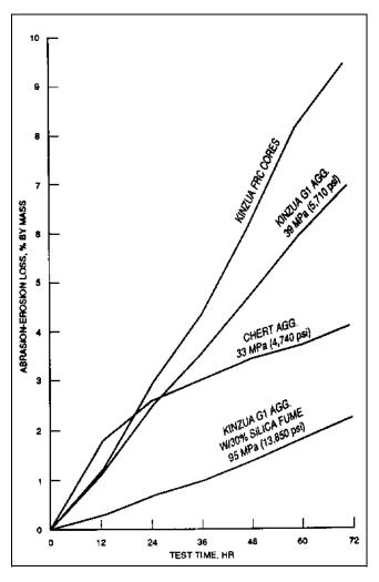
Figure 8-35. Results of selected abrasion-erosion tests. Kinzua Dam
