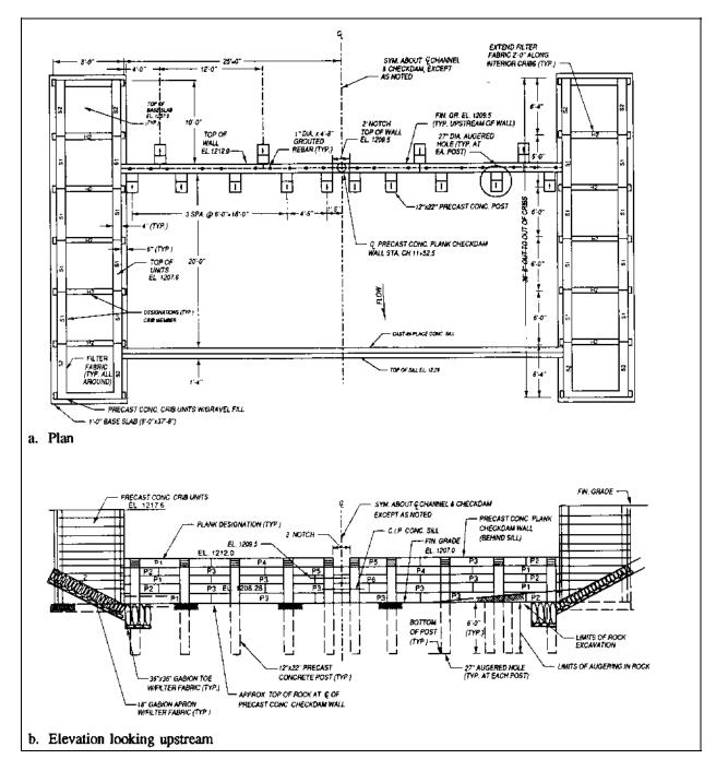
Figure 8-42. Structural plan and elevation, Chauncy Run Checkdam No. 2
