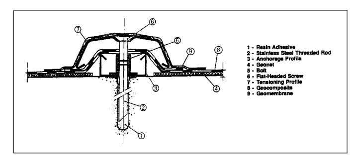
Figure 8-58. Detail of vertical anchorage and drainage profile
