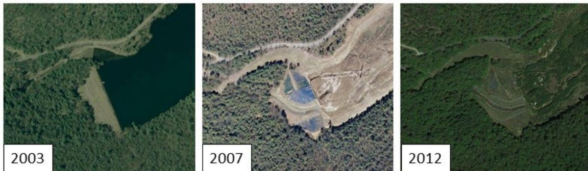
Figure 26. Aerial photographs of Birch Run Dam before, soon after, and 5 years after dam breaching.
