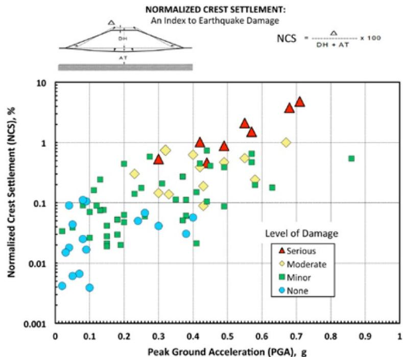
Figure 4-3: Settlements and Damage for Embankment Dams during Earthquake-excluding liquefaction settlement (Swaisgood, 2014)
