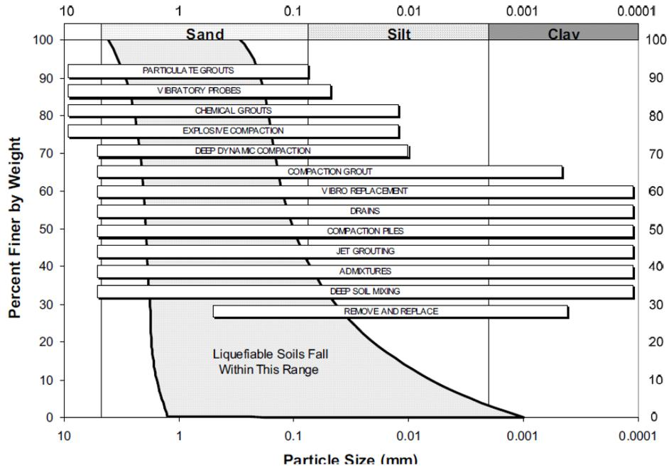
**Figure 4-14: General applicability of ground improvement methods for liquefiable soils**
