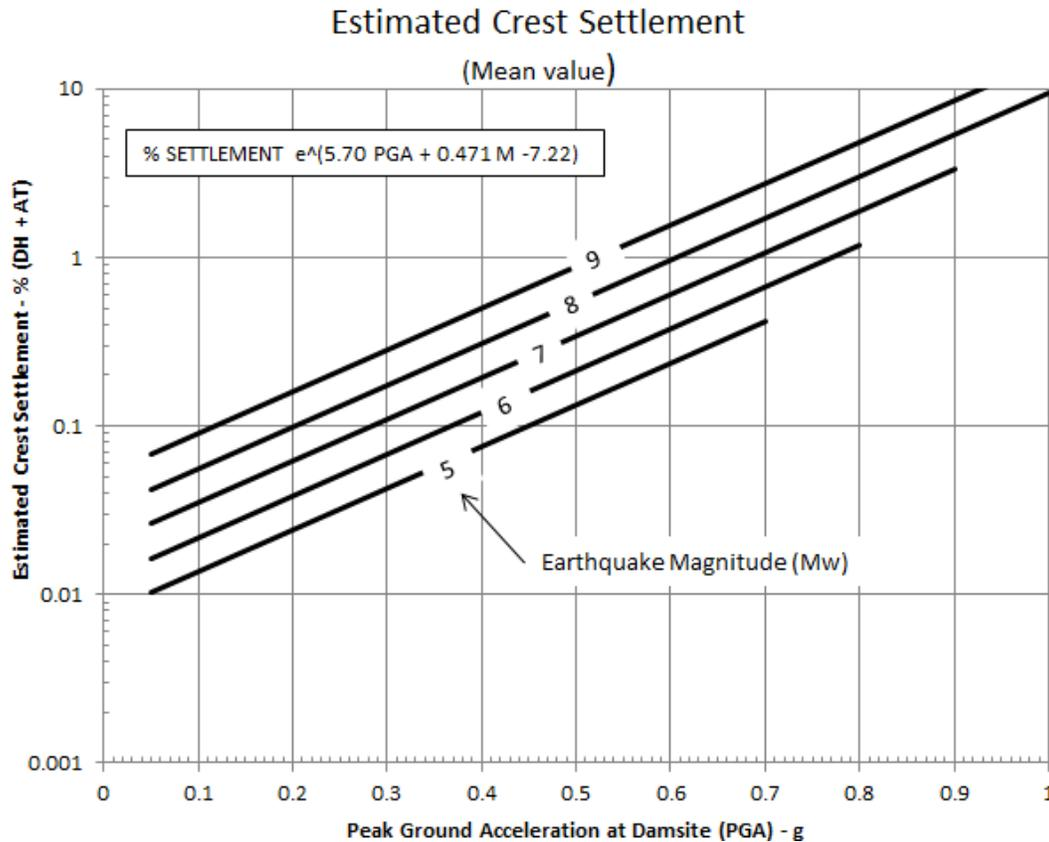
**Figure 4-13: Predicted normalized crest settlements of dams** (from Swaisgood, 2014)
