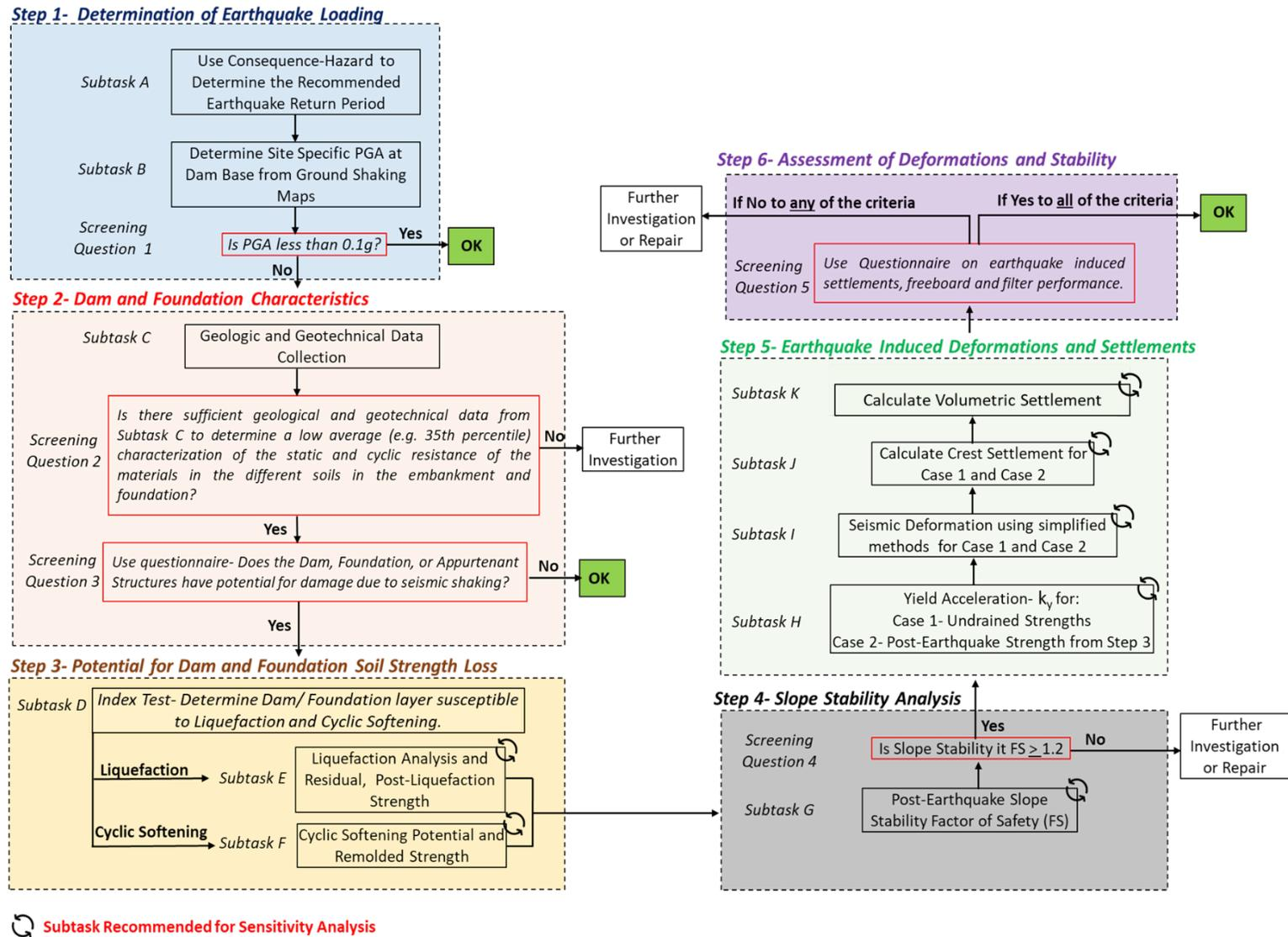
Figure 4-1: Simplified Seismic Analysis
