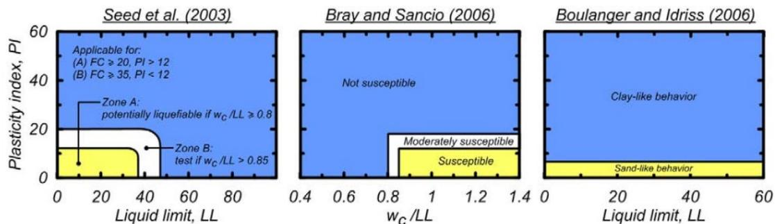
**Figure 4-5: Methods used to determine liquefaction susceptibility: Seed et al. (2003); Bray and Sancio (2006); and Boulanger and Idriss (2006).**
