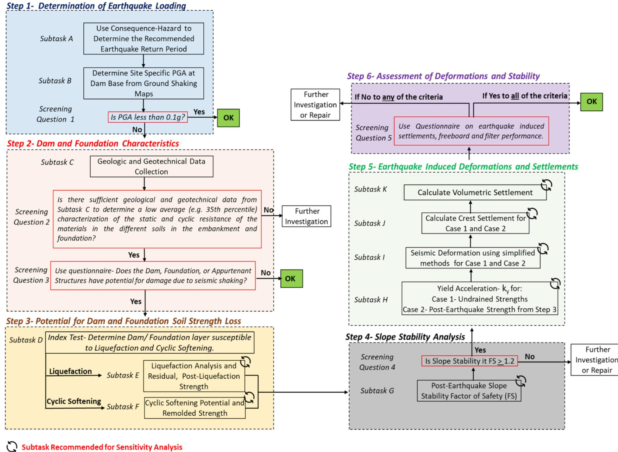
Figure B-1: Simplified Seismic Analysis Procedure
