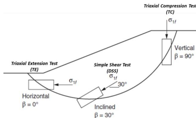
**Figure 4-10: Stress orientation at failure and undrained strength anisotropy of clays**
