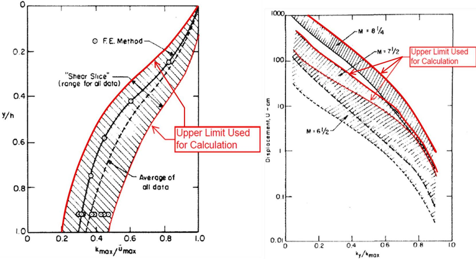
Figure 4-12: a) Variation of "Maximum Acceleration Ratio" with depth of sliding mass; b) Variation of predicted displacement ( $U$ ) with  $K_y/K_{max}$  ratios (Figures from Makdisi and Seed, 1977)
