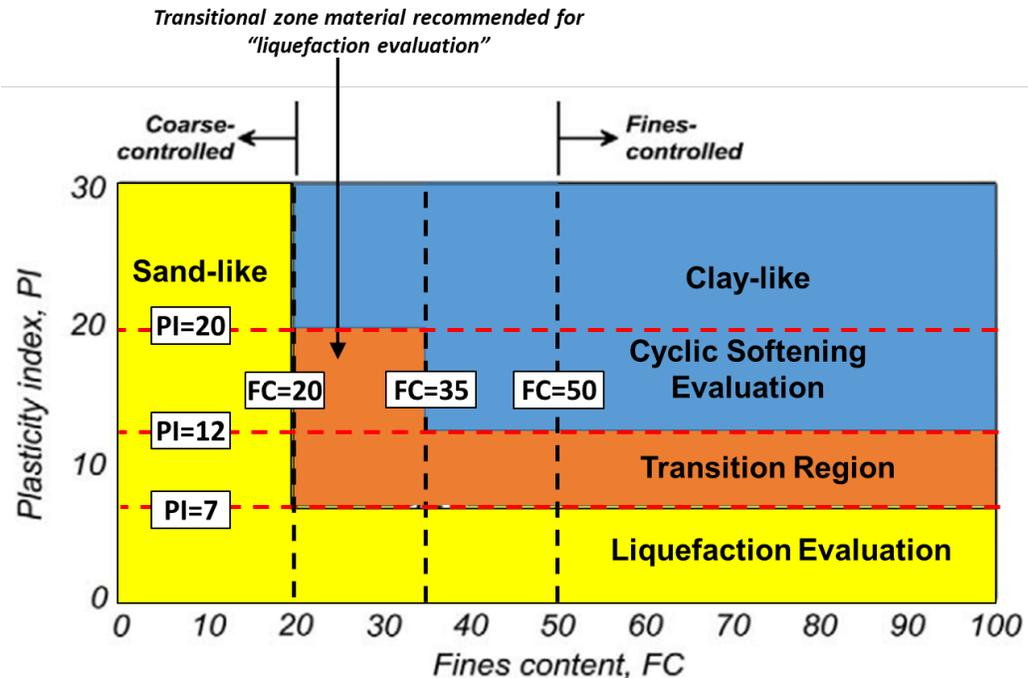
**Figure 4-6: Liquefaction susceptibility chart**
