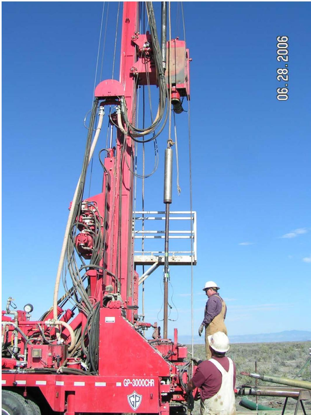
**Figure 12.8.3-1. Upper Colorado Region's Gus Pech rotary drill rig.**
