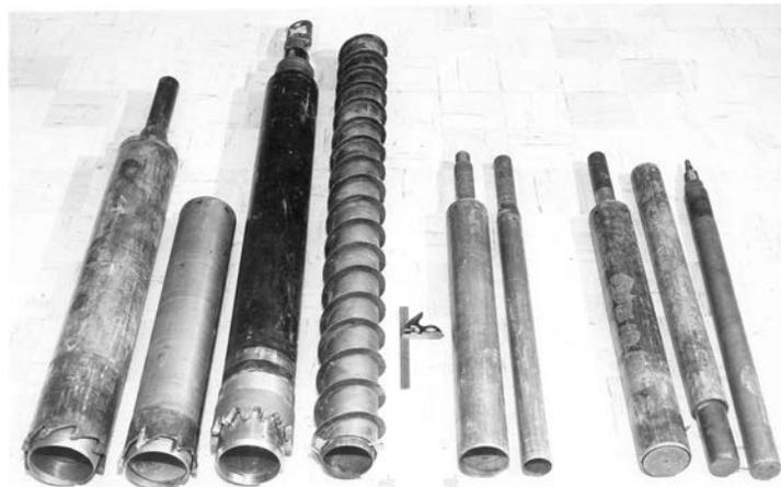
Figure 12.8.5-1. Several different types of soil samplers typically used in conjunction with hollow-stem augers.
