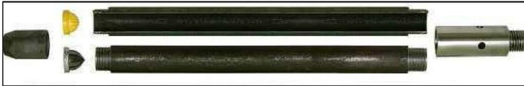
**Figure 12.14.1.1-1. View of a split-spoon SPT sample barrel.**
