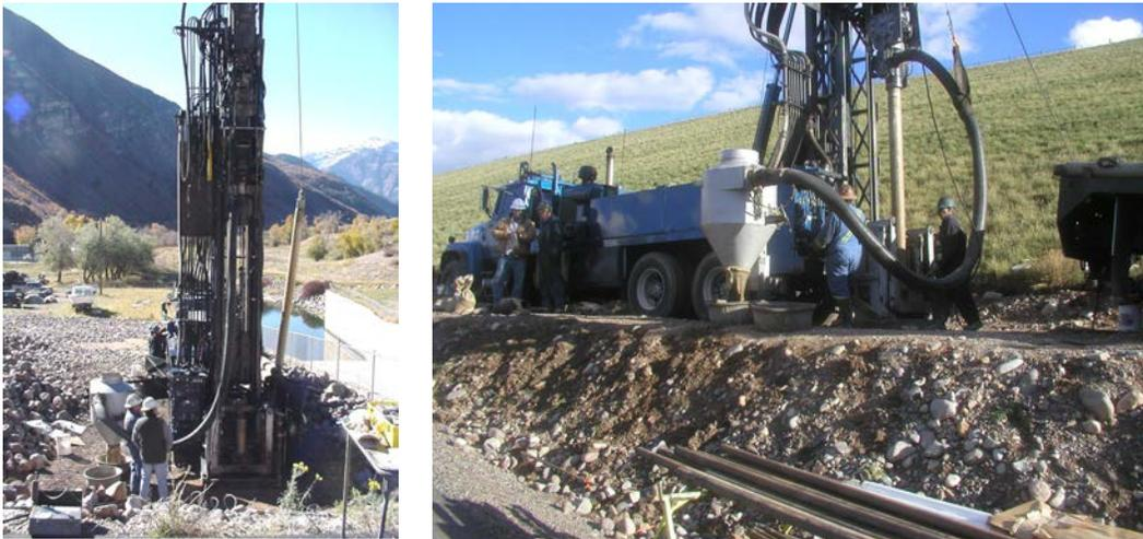
**Figure 12.8.7-1. Becker drill performing BPT in embankment and foundation materials.**
