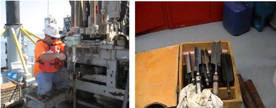
Figure 12.14.1.4-1. A vane shear test in progress using a drill rig to provide torque. Many sizes of vanes are available as shown in second photograph.
