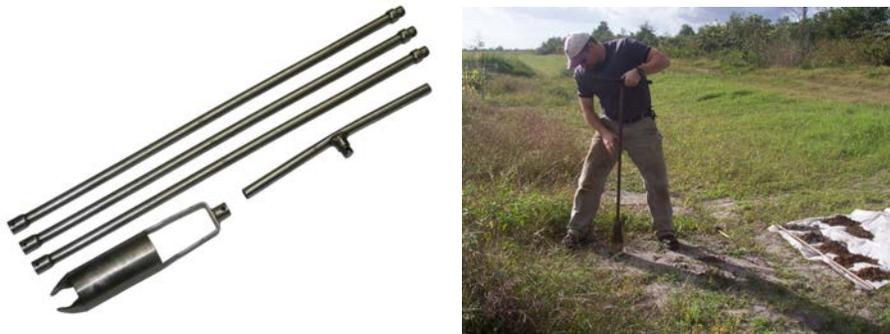
Figure 12.8.2-1. Typical hand augers used for soil sampling.
