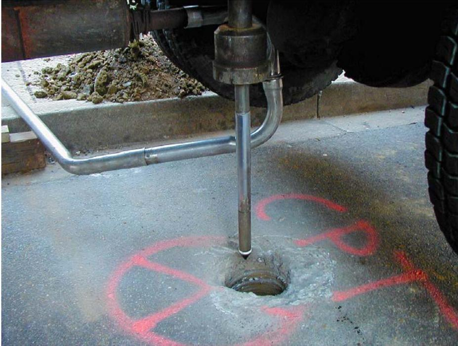
Figure 12.14.1.3-2 CPT probe being advanced through a “starter” hole.
