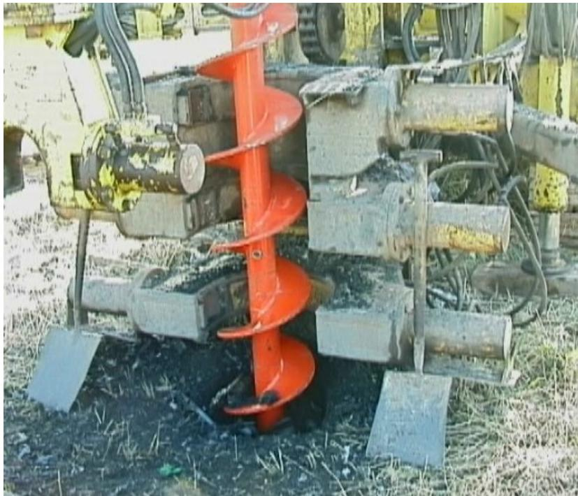
**Figure 12.8.2-2. Solid-stem flight auger.**
