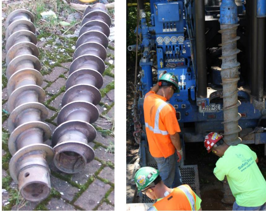
Figure 12.8.2-4. Hollow-stem flight augers are extensively used by Reclamation.
