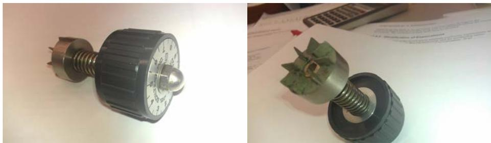
**Figure 12.14.1.9-1. View of TORVANE test shear device.**
